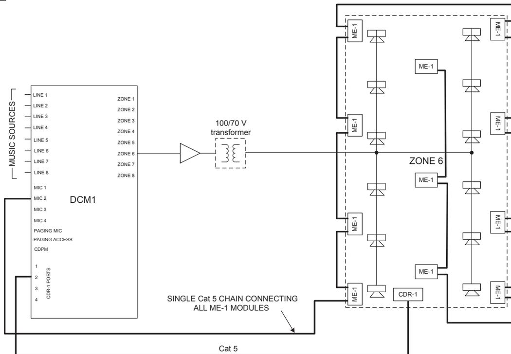
This example shows what might be a large hall or multi-purpose area forming one of the DCM1's zones (Zone 6 in this case). A single CDR-1 is fitted at one end to select and control the music routed to the area.
